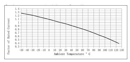
Operating Temperature: -40°C to +125°C, with proper rerating factor applied
