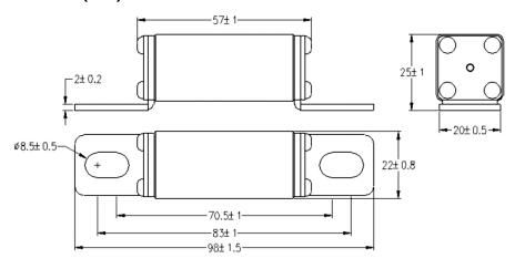
Note: Recommend tightening torque is 12+/-1.0Nm (M8)
