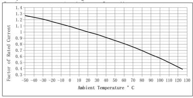
Operating Temperature:  $-40^{\circ}$ C to  $+125^{\circ}$ C, with proper rerating factor applied
