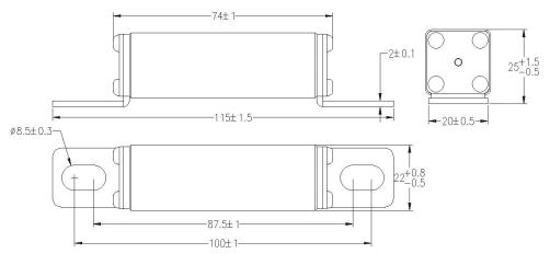
Note: Recommend tightening torque is 12+/-1.0Nm (M8)
