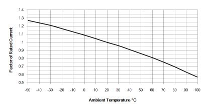
Operating Temperature:  $-40^{\circ}$ C to  $+100^{\circ}$ C, with proper rerating factor applied.
